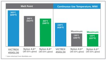
VICTREX PEEK 450GL30 valve components outperform 30% glass reinforced nylon mainly due to:
